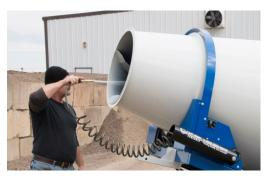
PORTAWASH SYSTEM is an on-board water system that provides water when none is available at the jobsite, enabling easy clean-up. It comes with a 23 gallon tank,; 25' perma-coil hose; 3.5 gal per minute pump with 45 P.S.I.
